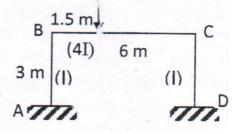
8. (a) Explain Kani's method of solving a frame subjected to sway forces. 4M(b) Evaluate the bending moment and shear force diagrams of a beam in figure by the Kani's method 6M
